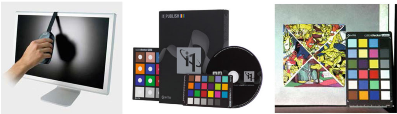
Fig. 19.2 Calibration process of optical devices
